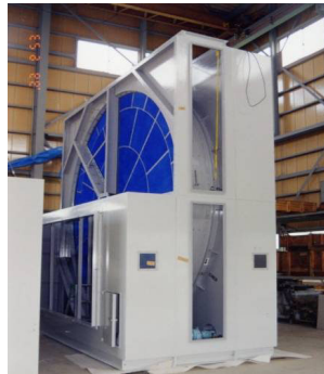
蜂巢狀沸石濃縮轉輪 Honeycomb type zeolite wheel concentrator
